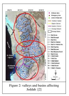
connect the city with 15 valleys starting with the valley of villages and Alasla in the north and up to the valley of Alkhomra in the south, some converge to form a main valley penetrating the city, and divided drainage basins affecting the city With three sections north, center and south [2].
